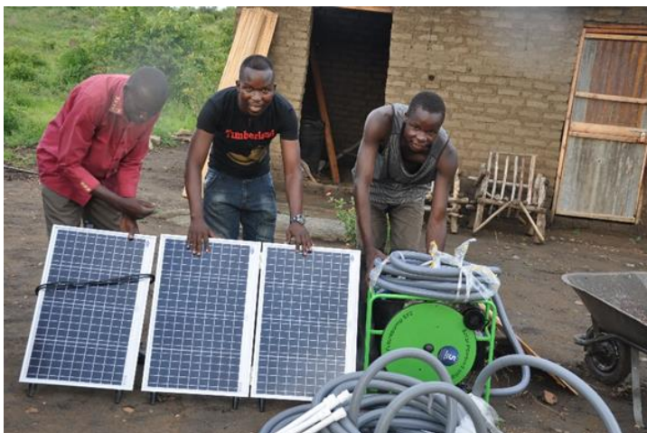
(Above)-The Solar panels used for irrigation
